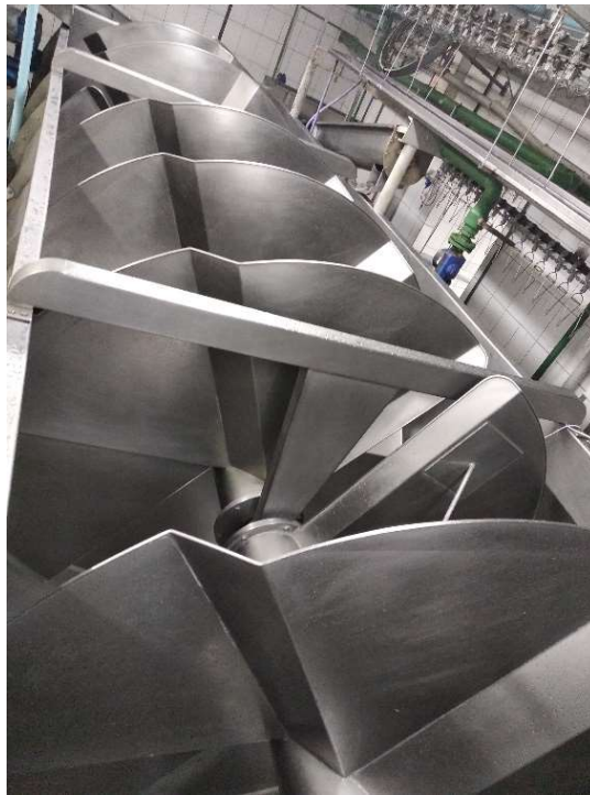
Figura 18: Pre-chiller e chiller
